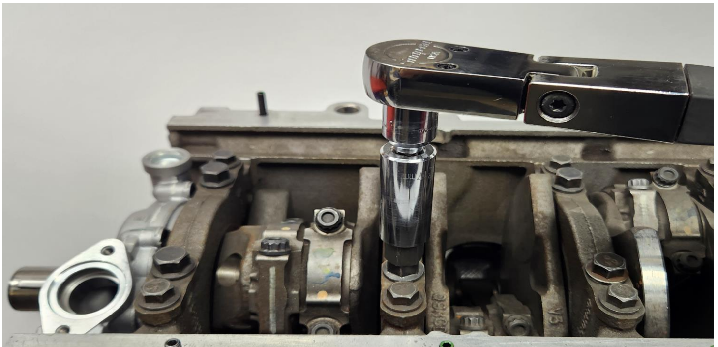
Step 7: Torque the standoff to 25 N-m
