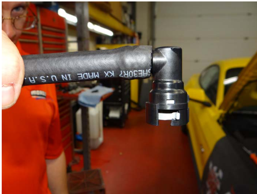
Step 10: Insert 90 degree fittings into one end of each hose provided in kit.
