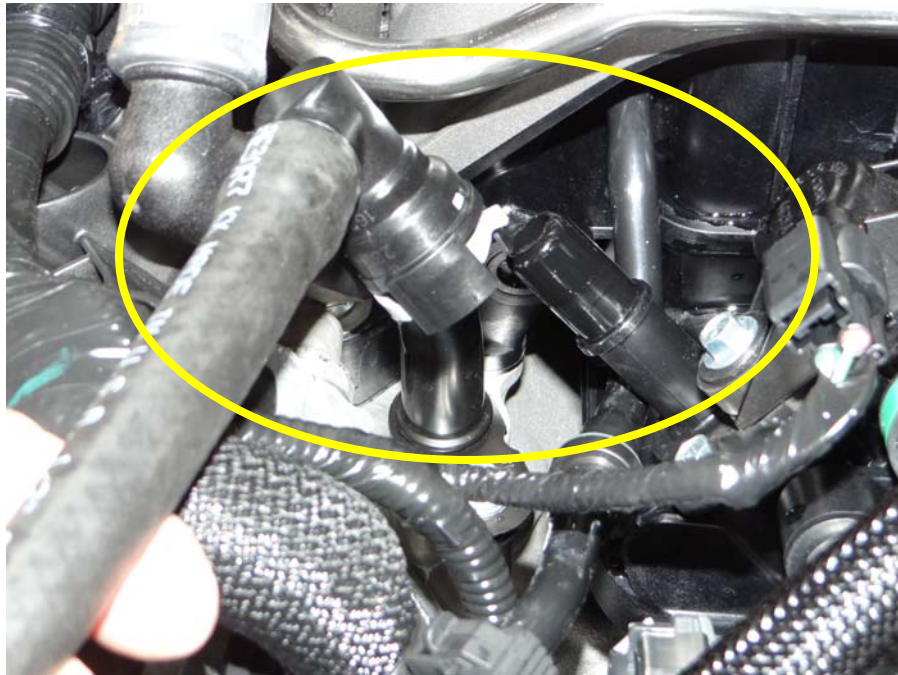
Step 11: Install (1) 90 degree fitting to intake nipple.
