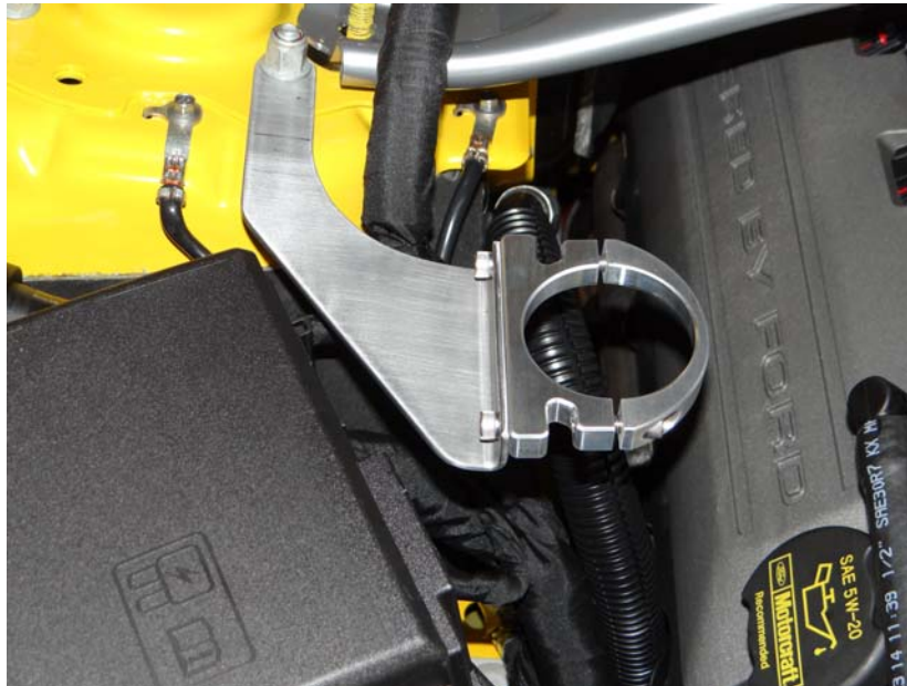
Step 16: Assemble clamp assembly to stainless steel mounting bracket using (2) 1/4-20x5/8 SHCS. Make sure reliefs are facing down.
