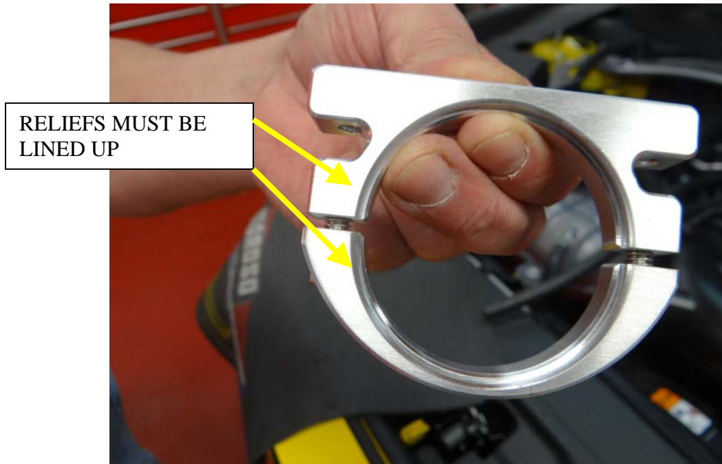
Step 15: Assemble billet clamp to billet saddle using (2) 1/4-20x5/8 SHCS.
