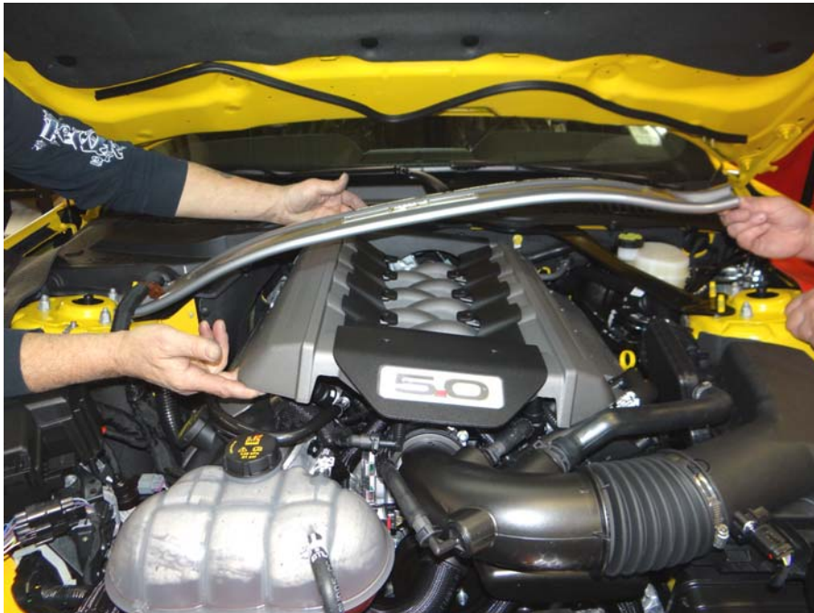
Step 4: Raise strut tower brace to allow engine cover to be removed.
