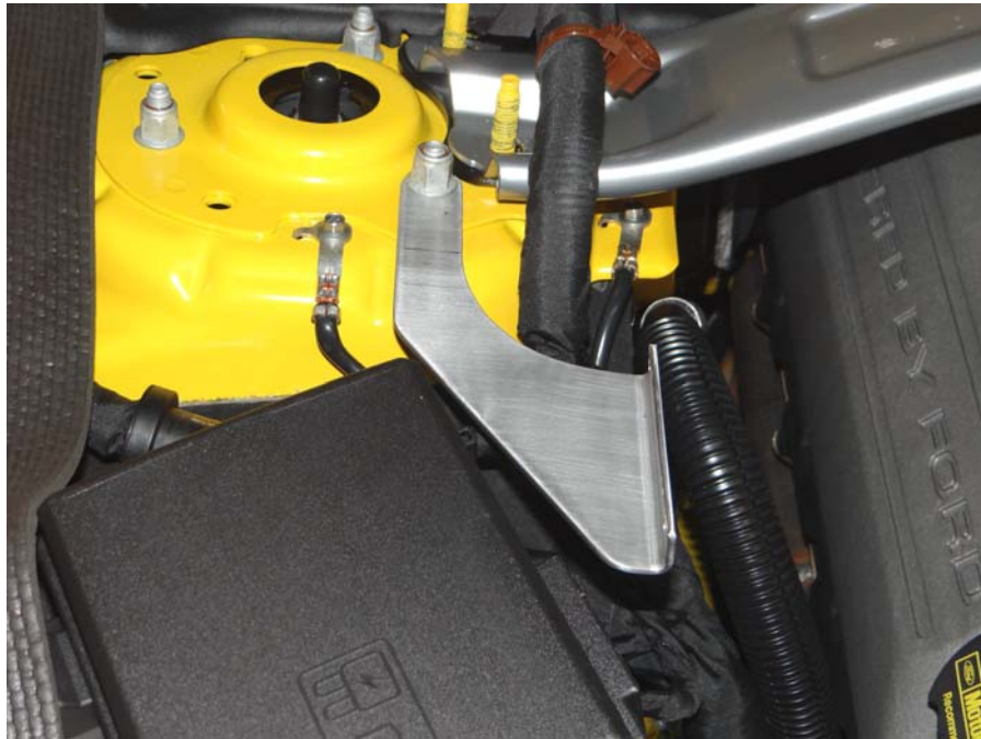
Step 14: Install stainless mounting bracket as shown.
