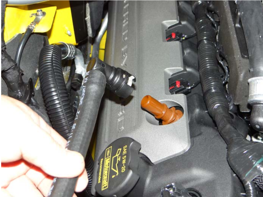
Step 12: Install 2 nd 90 degree fitting to valve cover nipple.
