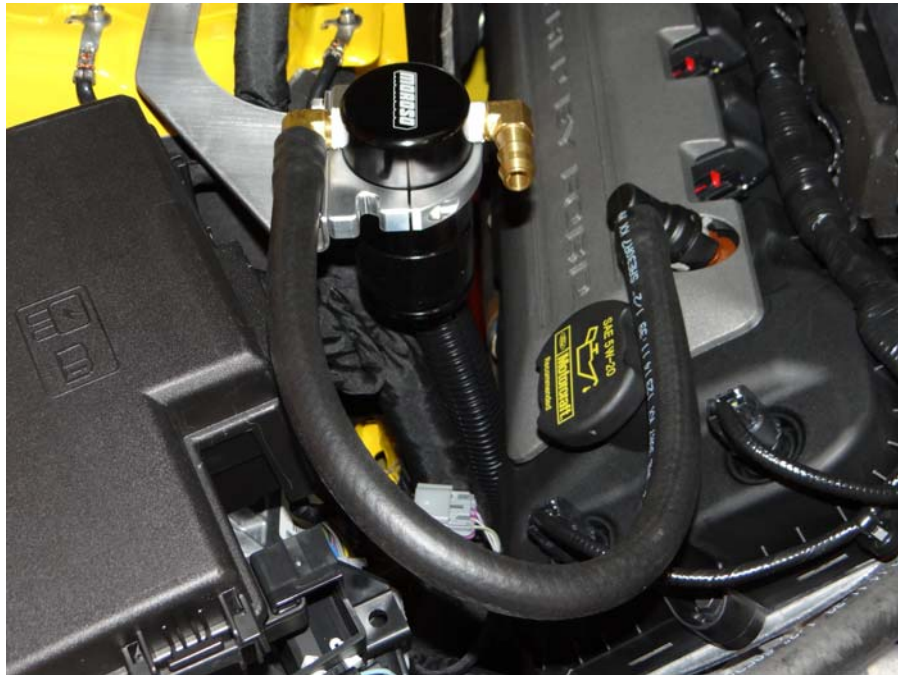
Step 20: Install hoses to air oil separator as shown.
