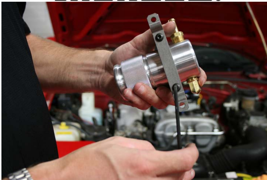
Step 3: Assemble billet clamp and stainless mounting bracket using (2) \frac{1}{4} x 20 x \frac{5}{8} BHCS
