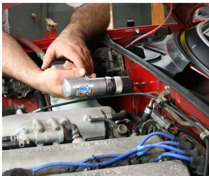
Step 7: Drill first 1/4" hole at marked location
