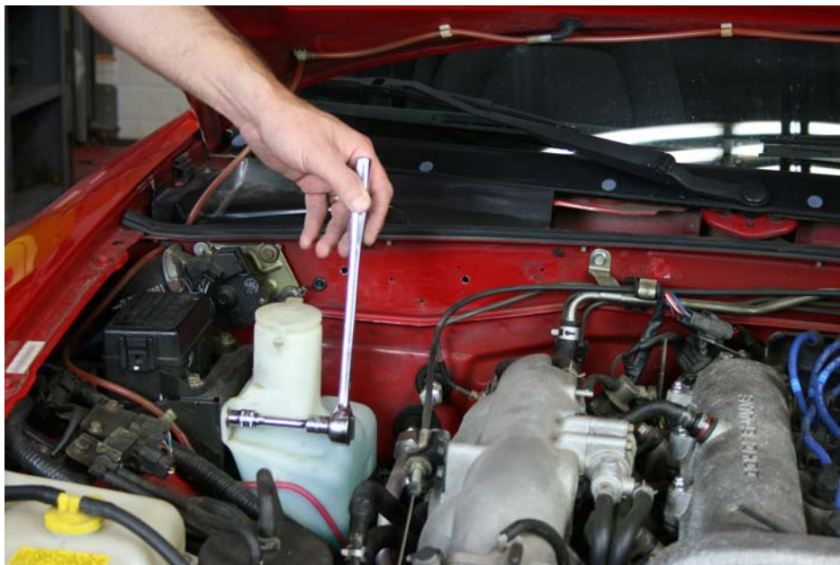
Step 9: Reinstall windshield washer tank mounting bolts
