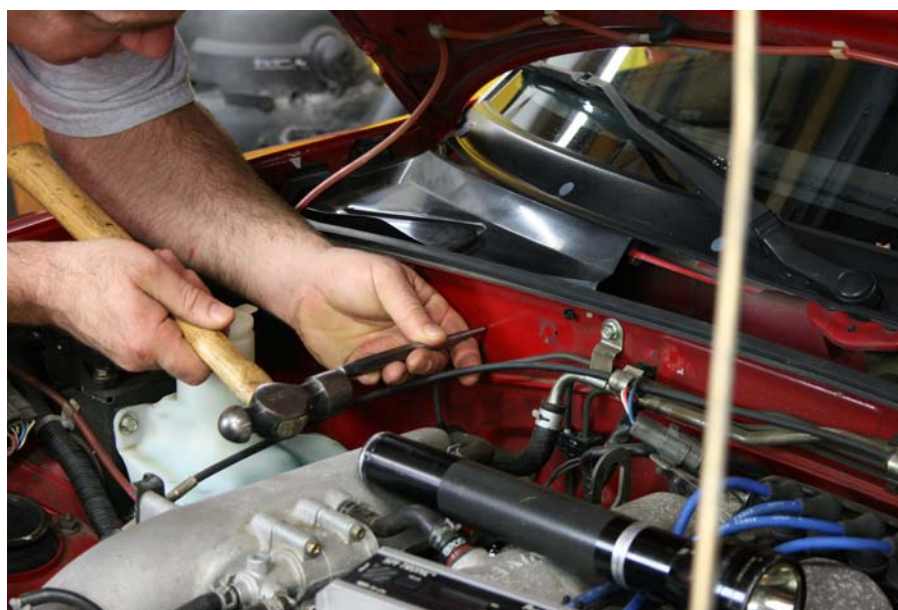
Step 5: Center punch hole locations previously marked
