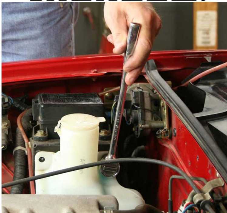
Step 6: Remove (2) mounting bolts from windshield washer bottle
