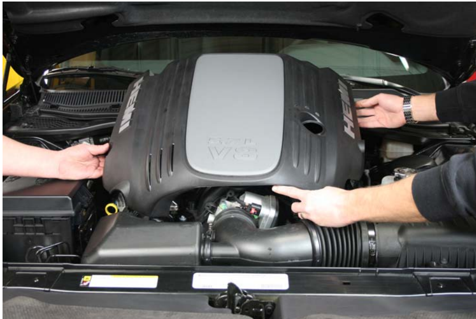
Step 1: Remove engine cover.
