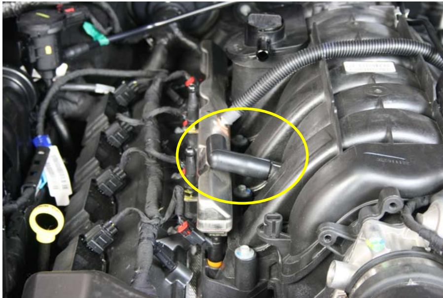
Step 3: Re-install 90 degree elbow in original location.
