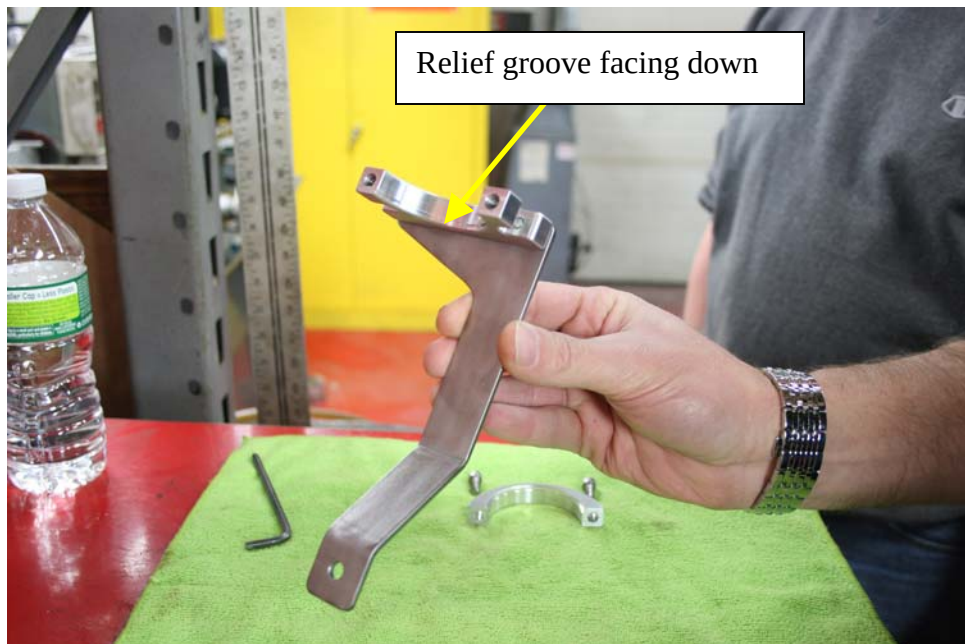
Step 5: Install clamp saddle to stainless mounting bracket using (2) ¼-20 x 5/8 SHCS.
